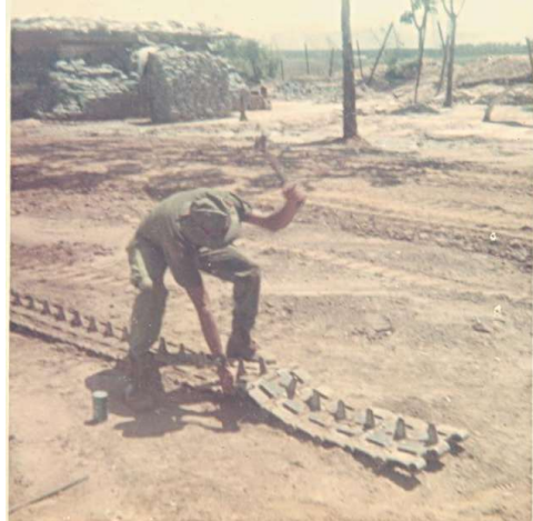
Jose replacing tracks.JPG (638x623)
